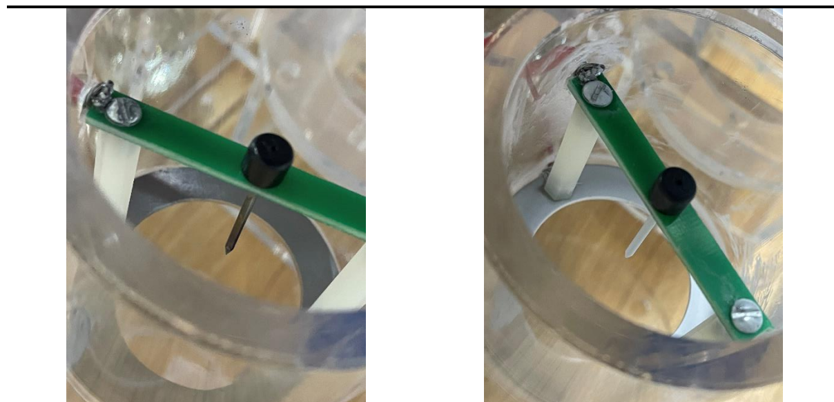
(a) Clean surfaces (b) Dirty (particle covered) surfaces Figure S21. Photos of charging pins before and after 30-day running.
