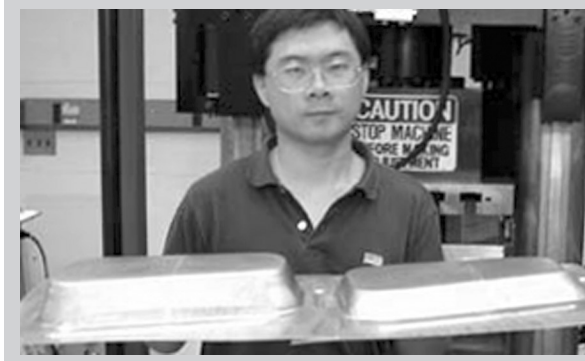
Figure 2. Ohio State University graduate student Jianhui Shang holds two pans stamped from automotive-grade aluminum. The pan on the right was stamped using traditional techniques. The one on the left was stamped using the same equipment, but using Glenn Daehn’s electromagnetic bump-forming technique. (Image courtesy of Ohio State University.)
