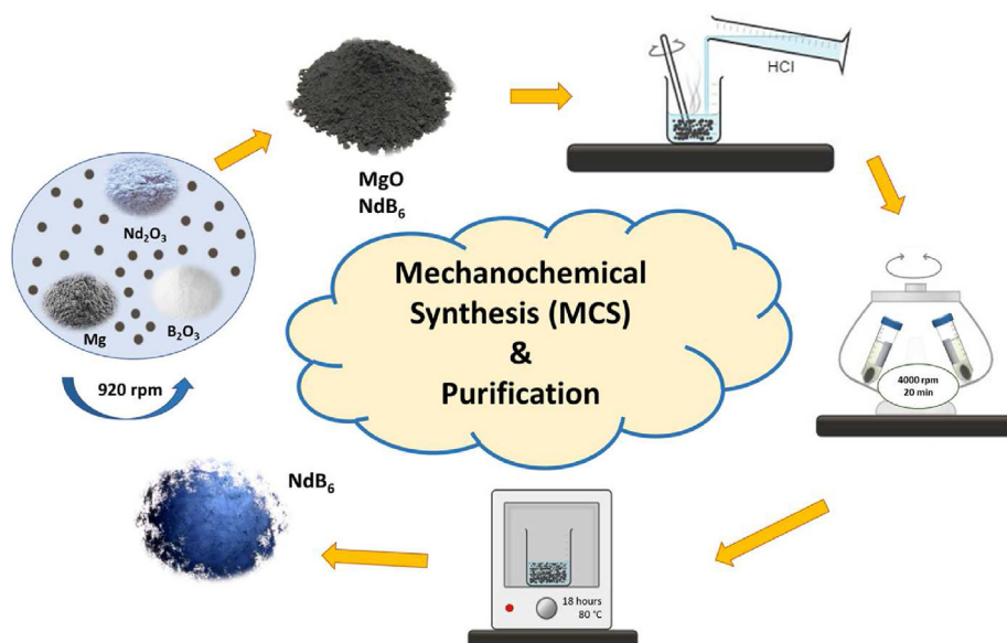
Fig. 1 – Schematic of synthesis procedure of \text{NdB}_6 powders.
